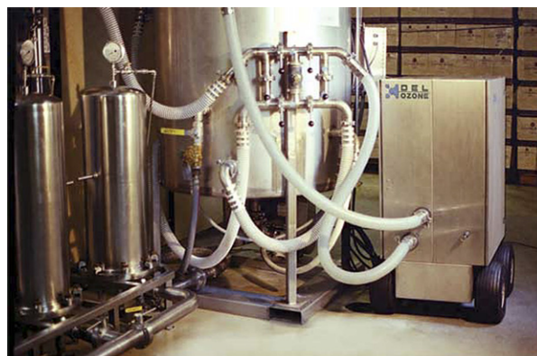
CIP systems using ozonated water. (courtesy of Del Ozone)
